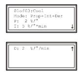
Choose which mode or actuator PID loop to tune, using the **01of03:** [Mode/Actuator name] setting.
